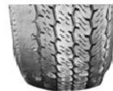
Signs of irregular tire wear
